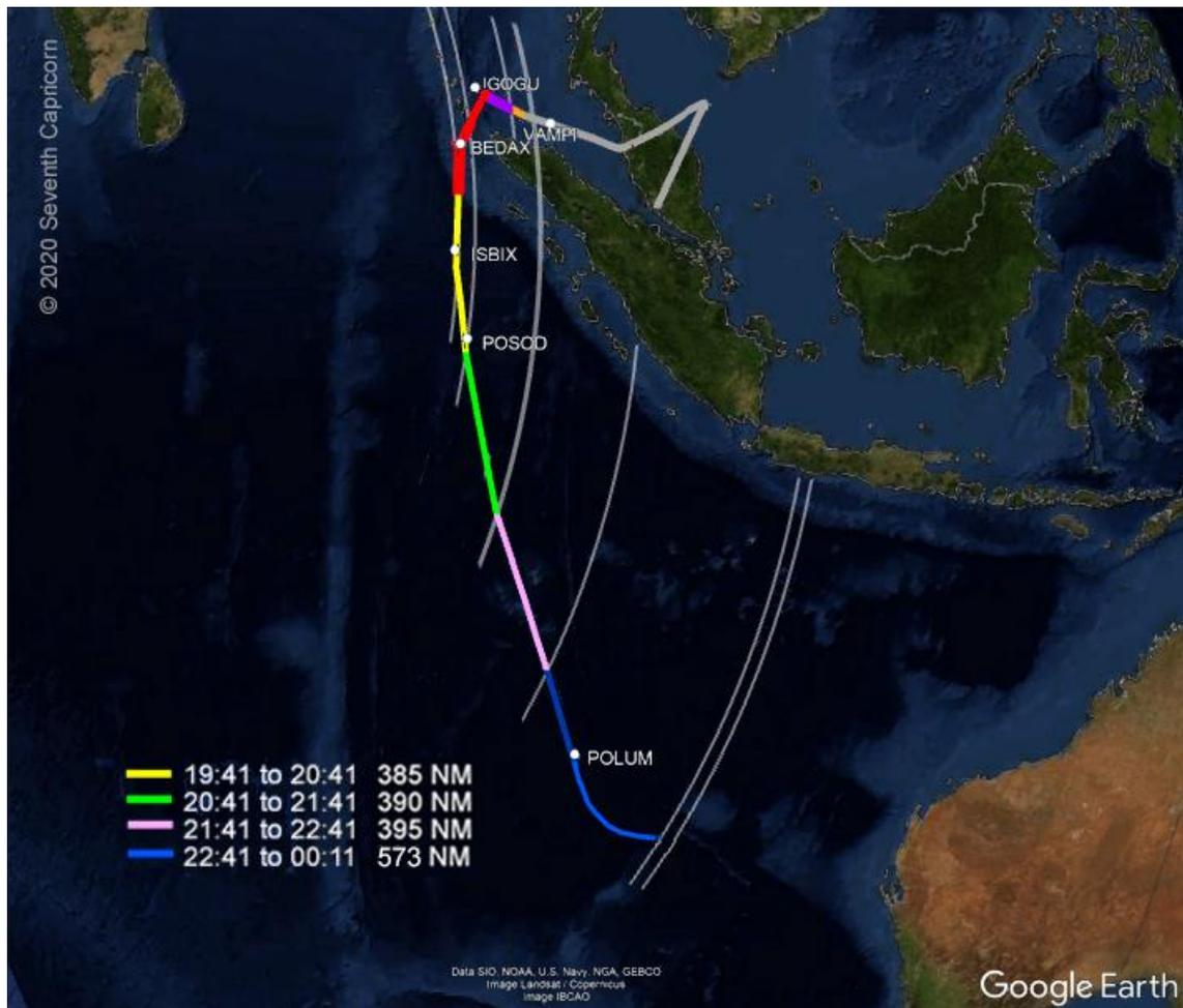
Figure 7. Reverse flight path plotted back from the 7<sup>th</sup> arc.
