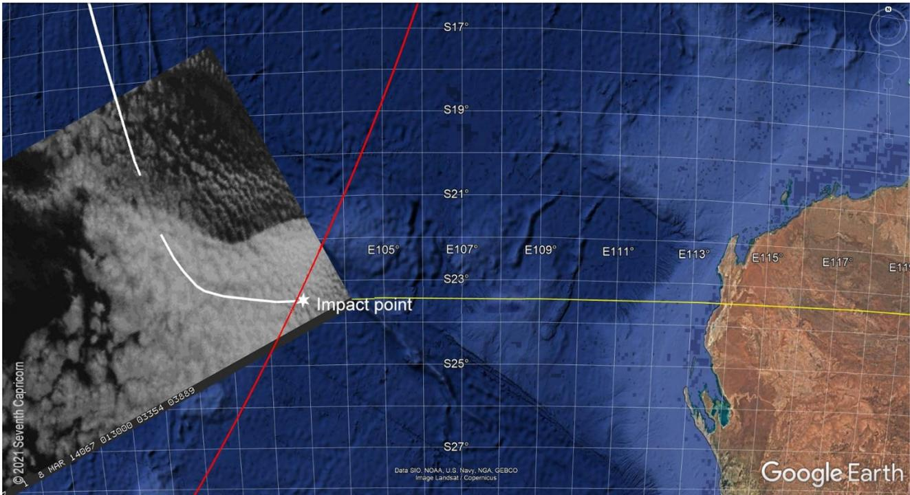
Figure 10. Enhanced satellite image with the reverse flight path (white) and 7<sup>th</sup> arc (red) overlay.
